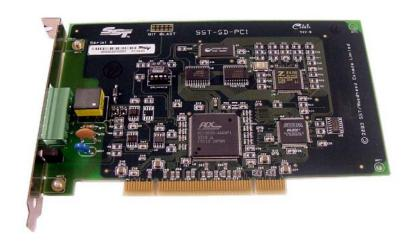
The SST Data Highway Plus interface card can connect your PCI bus computer to Allen-Bradley Data Highway Plus (DH+) and 1771 Remote I/O (RIO) (adapter or scanner mode) networks ▲
