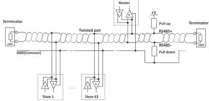
A daisy-chain (linear) topology and UTP/FTP cables are strongly recommended for multiple sensors. For proper operation of the interface, terminators (120 ohms resistors) must be installed at both ends of the bus. The device has a built-in 120-ohm resistor. To terminate the bus, the "RS485-" and "Term" terminals must be shorted.
