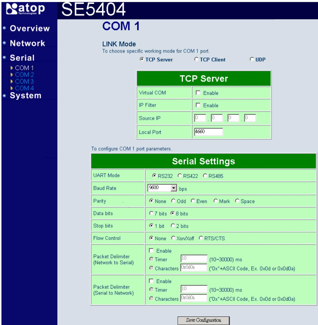
Figure 3.22 Com1 setup-TCP server
