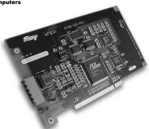
The SST Data Highway Plus interface card can connect your PCI bus computer to Allen-Bradley Data Highway Plus (DH+) and Remote I/O (RIO) (adapter or scanner mode) networks ▲
