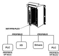
The BradCommunications SST PROFIBUS scanner fastens onto the side of any PLC-5 processor that supports a side car and functions with the Allen-Bradley PLC-5 as a co-processor.
