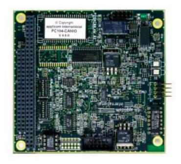
Based on a unique industrial communications concept, applicomIO® provides high-speed, deterministic communications between real-time applications (Open Controller, PC-based Control, Soft Logic, etc.) and various I/O modules communicating through fieldbuses.
