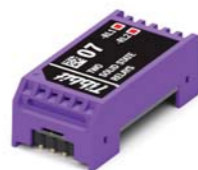
#07 Two solid-state relays
