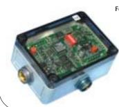
The Brad Harrison® Bus Extender extends the allowable trunk or drop line length of a DeviceNet system. The Bus Extender allows you to multiply cable lengths to increase drop lines, or can facilitate the creation of a star topology on the network. As an added benefit, the extender can isolate sections of the network from electrically *noisy* devices such as variable frequency drives or DC switching power supplies.
