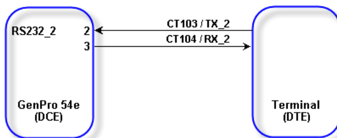
Figure 22 : Normalized signals of serial link RS232_2
