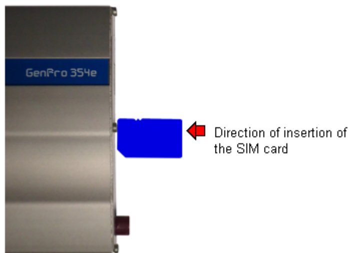
Figure 35 : Installation of the modem
