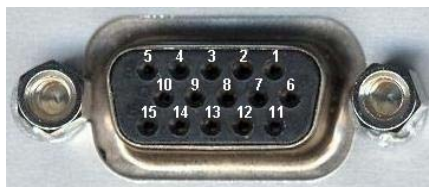
Figure 7 : 15-pin Sub D HD connector
