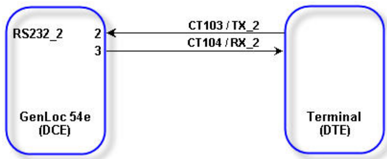
Figure 23 : Normalized signals of serial link RS232_2
