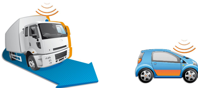
Figure 44 : Installation of GPS antenna not recommended
