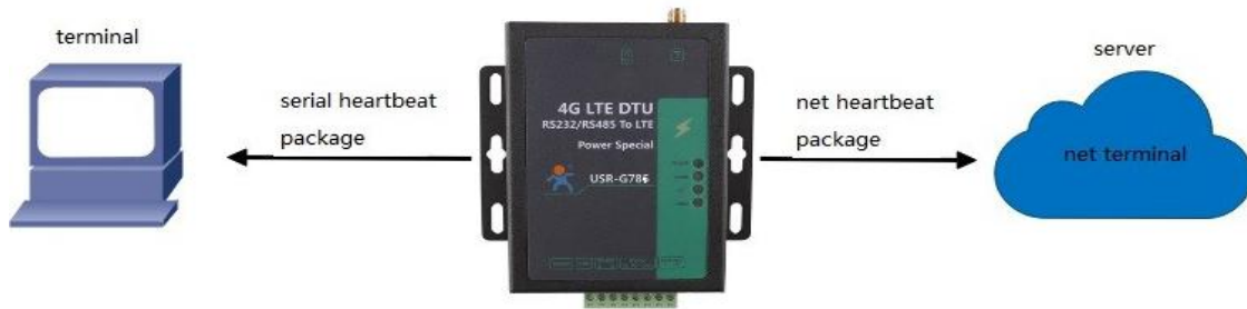
Diagram 10 Heartbeat schematic diagram
