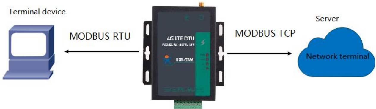
Diagram 15 Modbus protocol conversion schematic diagram
